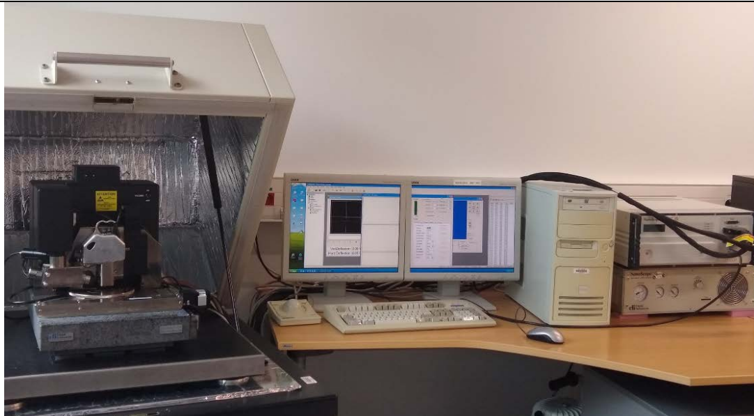
Figure 1-1: Complete Veeco Dimension 3100 AFM used in our study. The system is composed of three components: the AFM head with the piezo systems (on the left), the AFM controllers (on the right), and the computer system that runs the instrument. A compressor below the table is used to maintain the anti-vibration table beneath the AFM head system.
