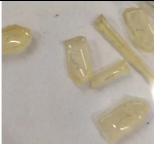
Figure 2-22: Roots embedded inside polymerized resin blocks. (Black thread like structures).
