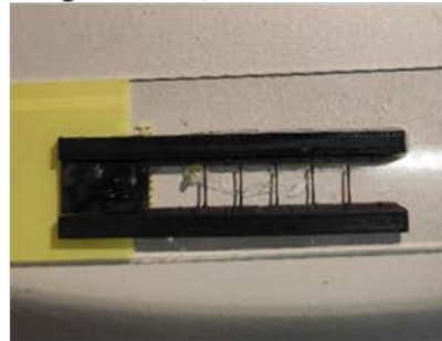
Resin made harp, quite brittle and light. Cannot confine root.
