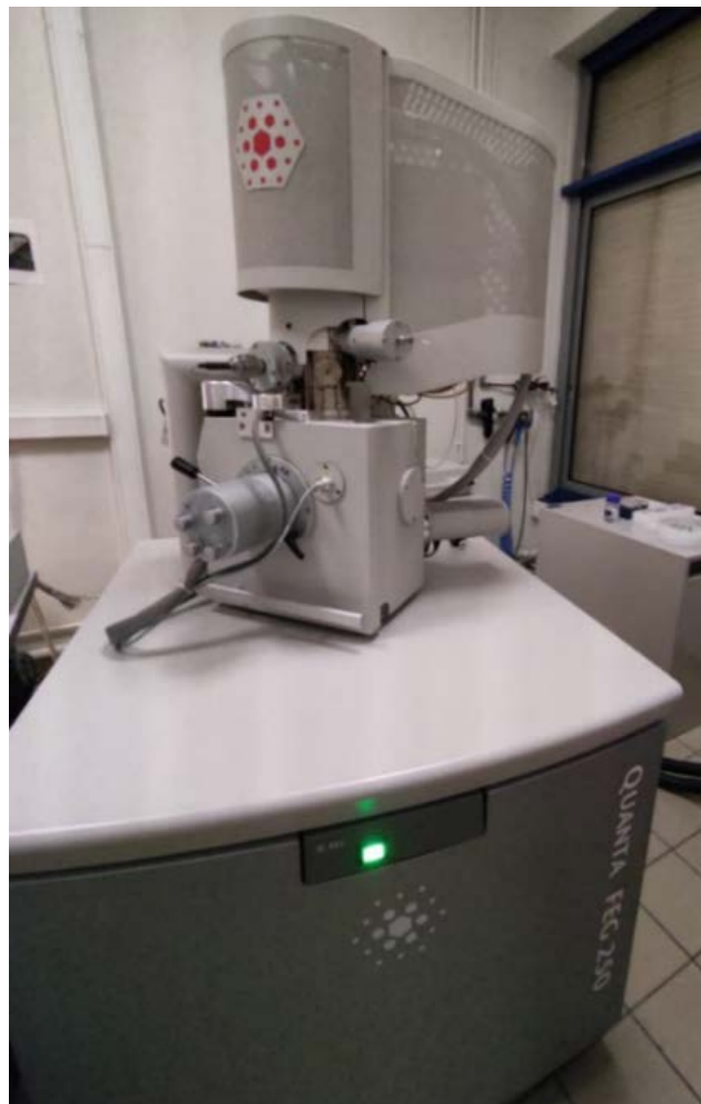
Figure 2-19: Quanta FEG-250 environmental SEM instrument used for high-resolution imaging at room temperature.
