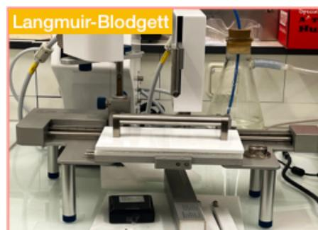
**Figure 26:** Langmuir-Blodgett trough used to prepare nanocube compact films.
