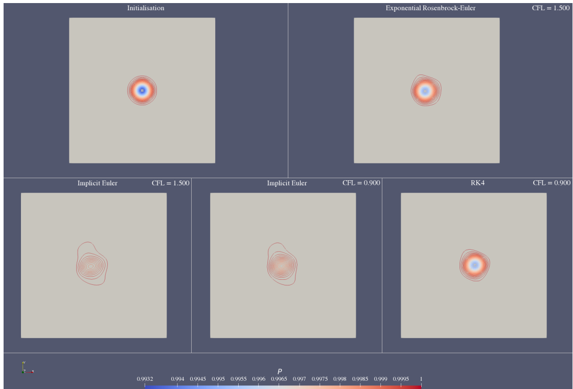
Figure 4.1: Initial solution (top left) and solution after one period for the exponential Rosenbrock–Euler method (top right), the implicit Euler method (bottom left and center) and the explicit RK4 method (bottom right). The first two simulations correspond to a CFL number of 1.5 whereas the last two to a CFL number of 0.9.
