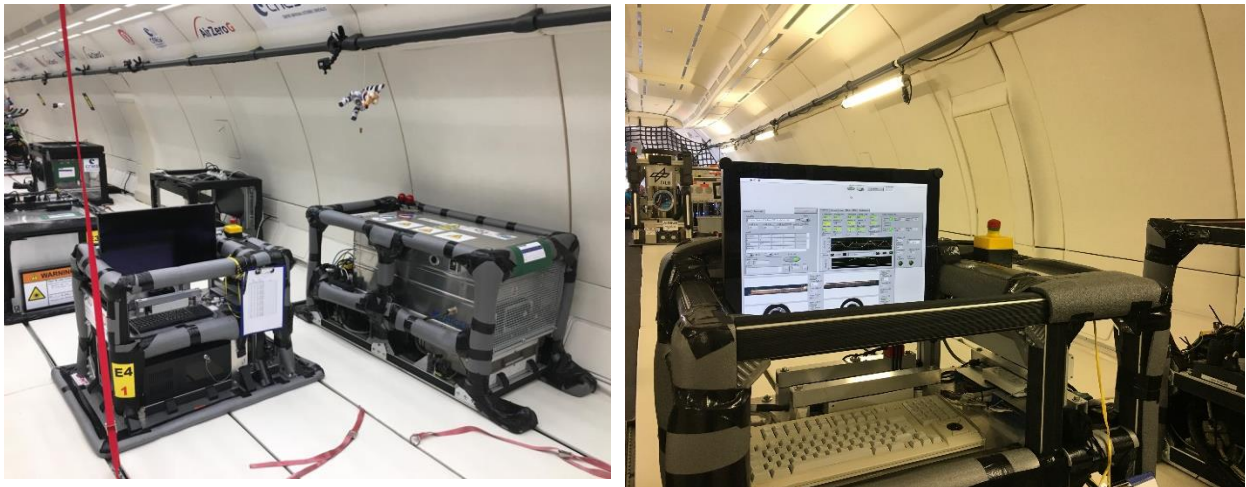
Figure E.1: The experiment inside the aircraft. The picture on the right is the control computer with the LabVIEW main interface during a simulation run test inside the Aircraft on the ground.
