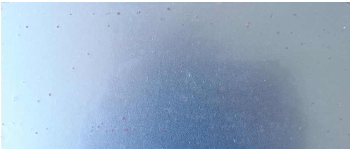
Figure 4.27: Surface aspect of a coating Co3-DMI after cure at 100°C for 1h30 and 160°C for 1h30 under vacuum, with DMI as the solvent.
