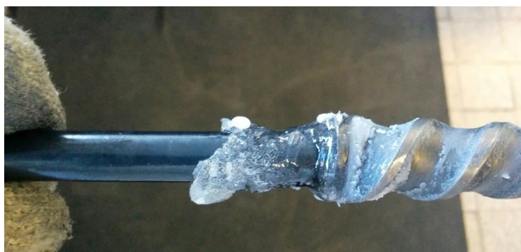
Figure 4.19: Clog of t-IPDI on one of the screws
