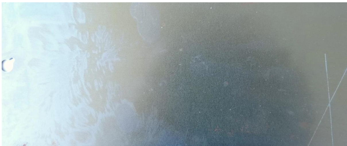
Figure 4.25 : Surface aspect of a coating Co1-MEK after cure at 100°C for 1h30 and 160°C for 1h30 under vacuum, with butan-2-one as the solvent.
