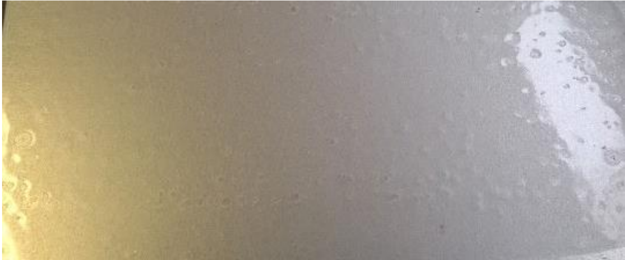
Figure 4.26: Surface aspect of a coating Co2-CPK after cure at 100°C for 1h30 and 160°C for 1h30 under vacuum, with cyclopentanone as the solvent.
