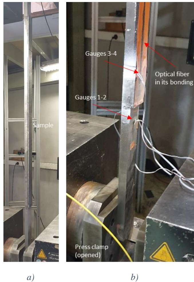
Figure 5.1-3: a) Initial tension test without instrumentation, b) Tension sample lower end with optical fiber and gauge instrumentation.
