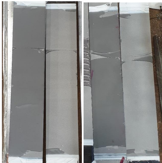
Figure A1-2: ENF failure mode without primer.
