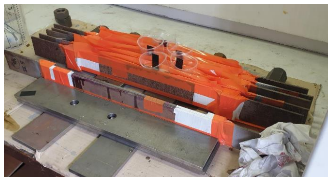
Figure 3.1-2: ENF Samples bonding.
