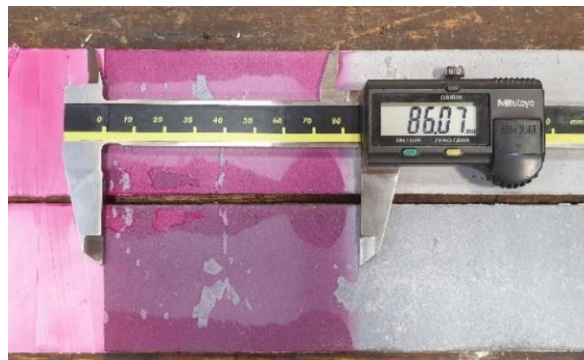
Figure 2.5-5: Visual measurement of the crack length at the end of the ENF test.
