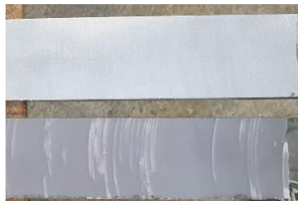
Figure 5.1-5: Adhesive failure and crack front shape of the samples.
