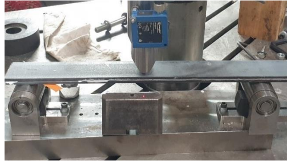
Figure 2.3-2: Photo of the ENF sample and ENF test bed.
