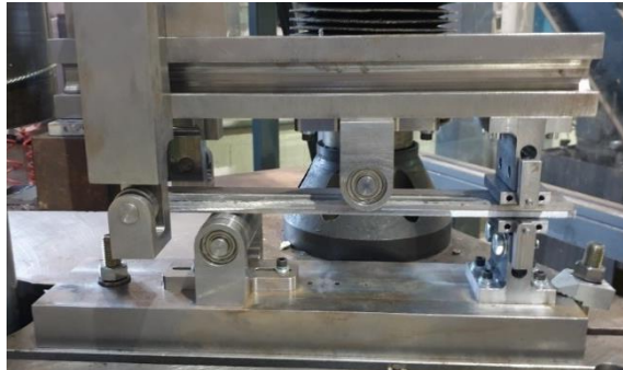
Figure 2.3-3: Photo of the MMB sample and MMB test bed.
