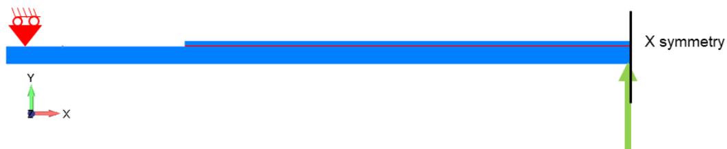
Figure 5.2-3: Finite element model boundary conditions for bending test.
