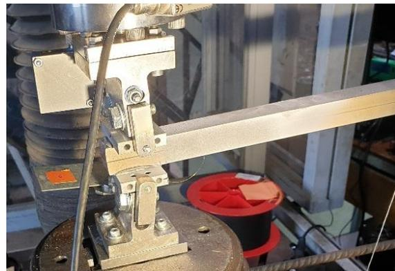
Figure 2.3-1: Photo of the DCB sample and DCB test bed.
