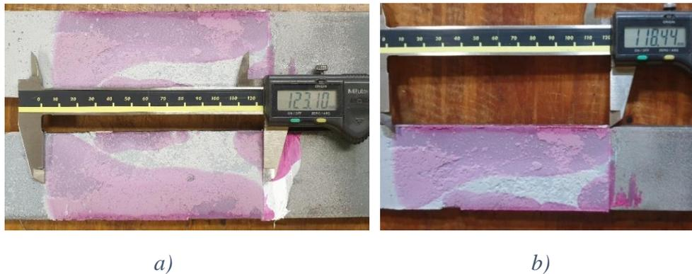
*Figure 2.4-4: Visual measurement of the crack length of the DCB test, a) in the middle and b) at the border.*
