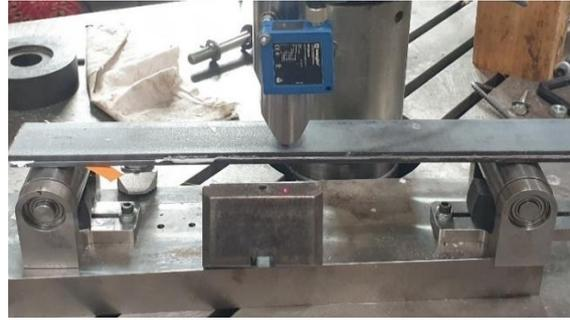
Figure 2.3-2: Photo of the ENF sample and ENF test bed.
