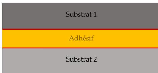
FIGURE 1.1 – Principe du collage structural
