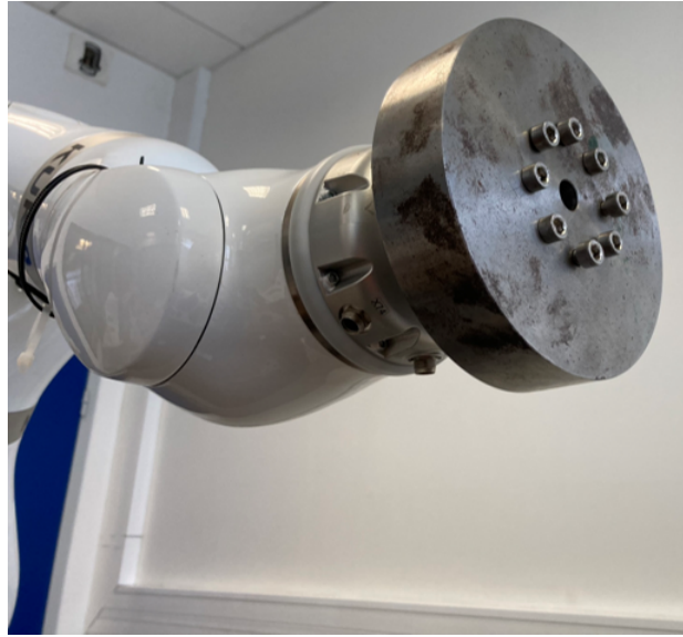
Figure B.3: Steel cylinder fixed to the tip of the robot used as payload.
