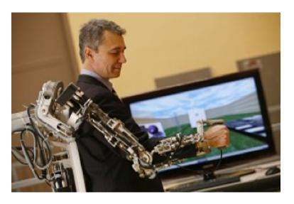
Figure 2.4: Photo of the exoskeleton ABLE worn by P. Garrec (credit to CEA-LIST) (Garrec, 2010)
