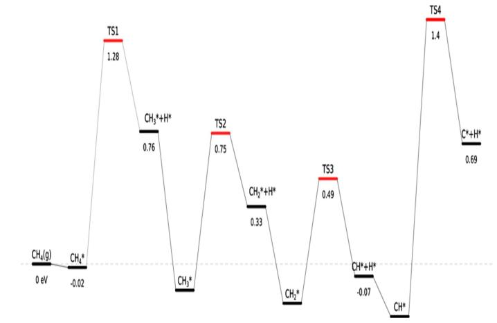
Figure 15 Activation energy profile for CH<sub>4</sub> dissociation steps.
