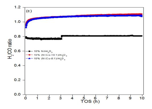
**Figure 31**  $H_2$ /CO ratio for DMR on Ni (111) and different Ni-Cu modified catalyst. Medium Ni-Cu catalyst (in blue) is showing sustained conversion over TOS of 10 h reprinted with permission from our research group.
