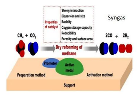
Figure 1 Summary of catalyst properties for DRM catalyst design modified from<sup>30</sup>.
