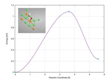
**Figure 21** Activation energy profile of CH oxidation by OH.OH is effective oxidant that helps skipping CH dissociation. Gray frame is showing T.S. configuration where OH is adsorbed on Top<sup>Cu</sup> while CH adsorbed on Top<sup>Ni</sup>.
