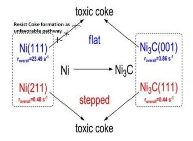
**Figure 6** Deactivation scheme to show schematically the phase transformation and coke formation adapted from <sup>37</sup>.
