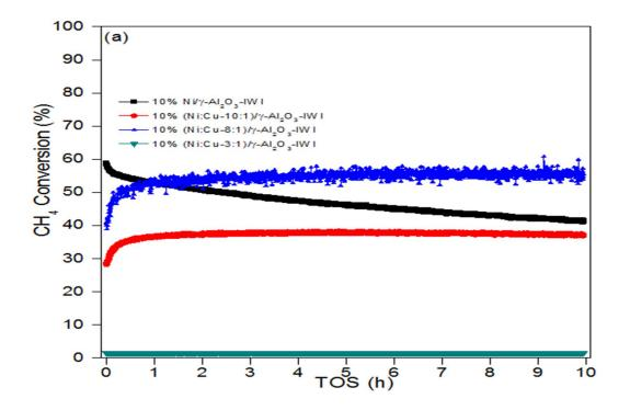
**Figure 29** CH<sub>4</sub> conversion for DMR on Ni(111) and different Ni-Cu modified catalyst. Medium Ni-Cu catalyst (in blue) is showing sustained conversion over TOS of 10 h reprinted with permission from our research group.
