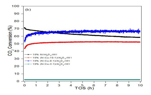
**Figure 30** CO<sub>2</sub> conversion for DMR on Ni(111) and different Ni-Cu modified catalyst. Medium Ni-Cu catalyst (in blue) is showing sustained conversion over TOS of 10 h reprinted with permission from our research group.
