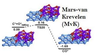
**Figure 9** Energy profile of C oxidation by lattice oxygen in FeO/Ni  $(1 \ 1 \ 1)$  (in unit of eV). The gray and red balls denote the C and O atoms, respectively adapted from <sup>67</sup>.
