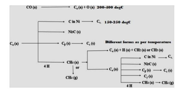
Scheme 1 Mechanism of carbon formation at the catalyst surface adapted from <sup>18</sup>.
