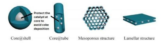
Figure 7 Categories of the Catalysts with Encapsulated Structures adapted from<sup>49</sup>.
