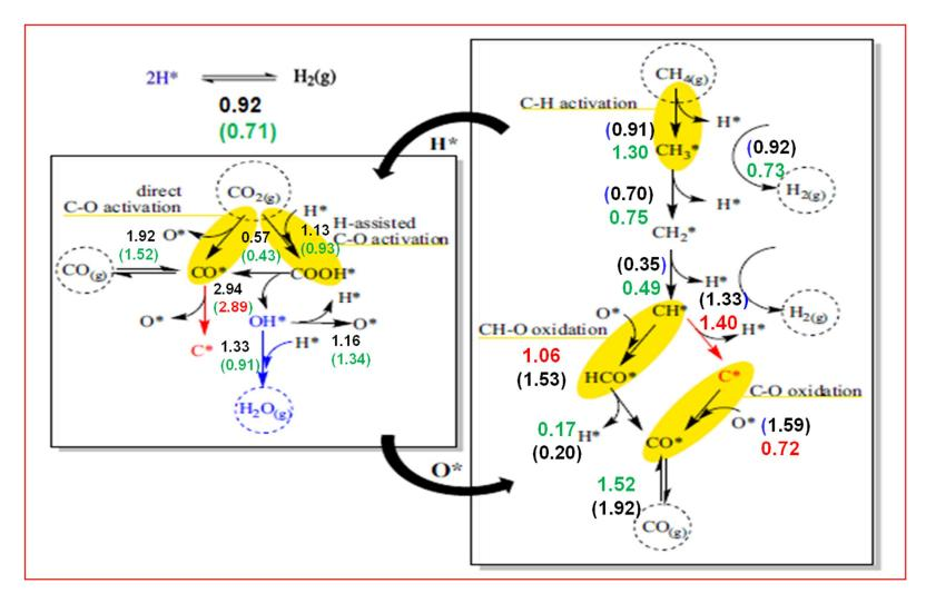
**Figure 28** Dominant pathways energy barriers in eV. For comparison,  $E_a$  in black is for Ni (111), green is for Ni<sub>2</sub>Cu surface while red color values are for carbon deposition/elimination steps on Ni<sub>2</sub>Cu surface adapted from <sup>119</sup>.
