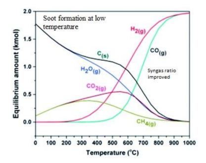
Figure 4.Equilibrium data for DRM process adapted from<sup>18</sup>.
