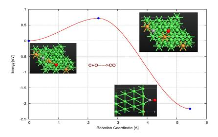
**Figure 19** Coke removal via atomic oxygen has smallest energy barriers of all other oxidation reactions. Black Frames are showing initial state, T.S. and final state.
