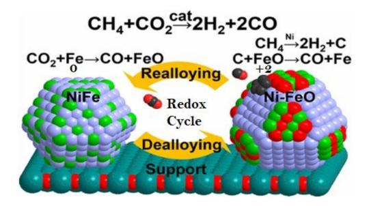
Scheme 3 Dealloying and realloying behavior of an Fe-Ni alloyed particle in DRM modified from <sup>66</sup>.
