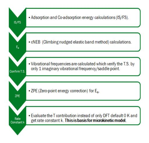
Figure 12 Sequence of DFT calculations shows workflow for DRM over Ni-Cu surface.
