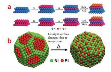
**Scheme 2 a)** Surface restructuring of Ni-Pt bimetallic systems induced by temperature and adsorbates; **b)** Evolution of the surface structure of Ni/Pt bimetallic nanoparticles upon thermal treatment adapted from<sup>55</sup>.
