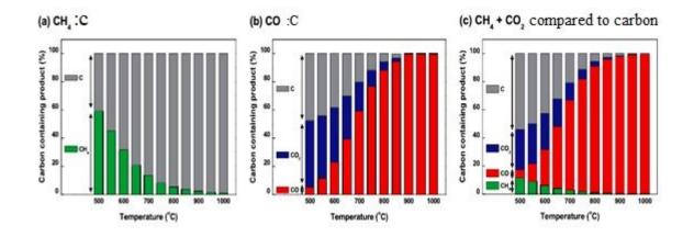
**Figure 3**.Carbon containing product for the catalytic reactions: (a) CH<sub>4</sub> decomposition (CH<sub>4</sub>=100%), (b) Boudouard reaction (CO=100%), (c) Dry reforming of methane (CH<sub>4</sub>=50% and CO<sub>2</sub>=50%) modified from<sup>30</sup>.
