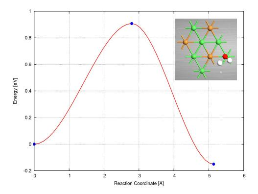
**Figure 24**  $H_2O$  formation via  $OH^*+H^*$  reaction. The weakly adsorbed  $H_2O$  may physically remove coke from catalyst surface in DRM elevated temperatures (steam). Gray frame is showing T.S.
