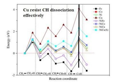
**Figure 10** The energy profiles for the dissociation of  $CH_4$  on elementary metals (Fe, Co, Ni and Cu) and bimetals (NiFe, NiCo and NiCu) surfaces modified from<sup>84</sup>.
