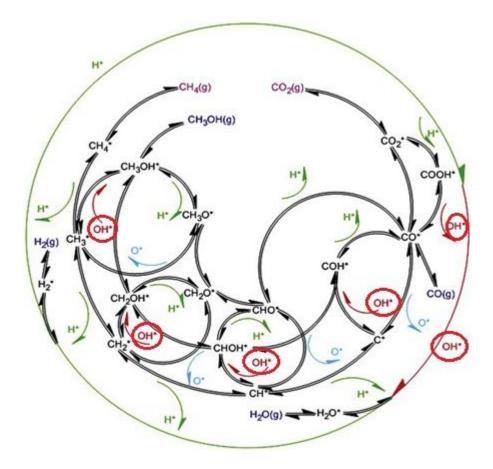
**Figure 5** Proposed mechanism for dry reforming of methane on Ni catalyst modified from<sup>33</sup> to show OH species role.
