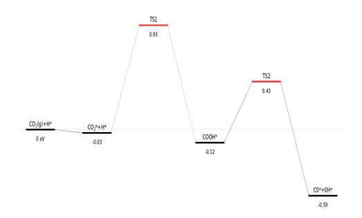
Figure 18 Activation energy profile for H-induced CO<sub>2</sub> dissociation.
