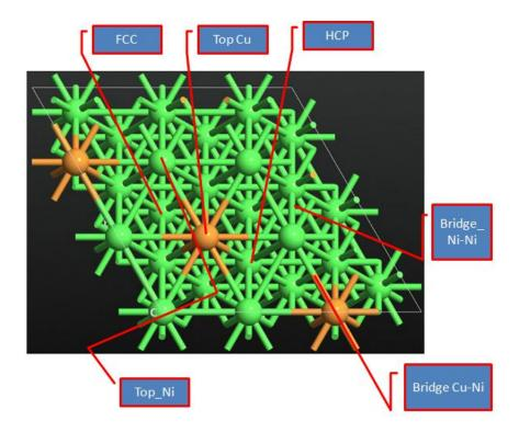
Figure 13 Ni<sub>2</sub>Cu overlayer of Ni (111).
