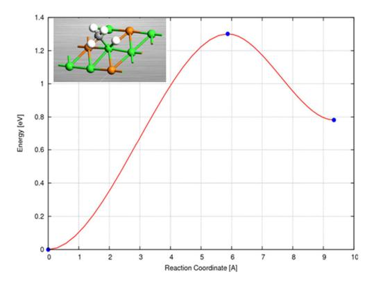
**Figure 14** Activation energy profile of  $CH_4$  dehydrogenation. Gray frame is showing T.S. configuration where  $CH_3$  and H are co-adsorbed on  $Top^{Ni}$ .
