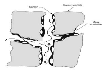
Figure 2 Pore plugging in a supported metal catalyst owing to carbon adapted from<sup>18</sup>.
