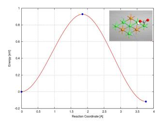
**Figure 17** Activation energy profile of H-induced CO<sub>2</sub> activation .Gray frame show T.S. configuration
