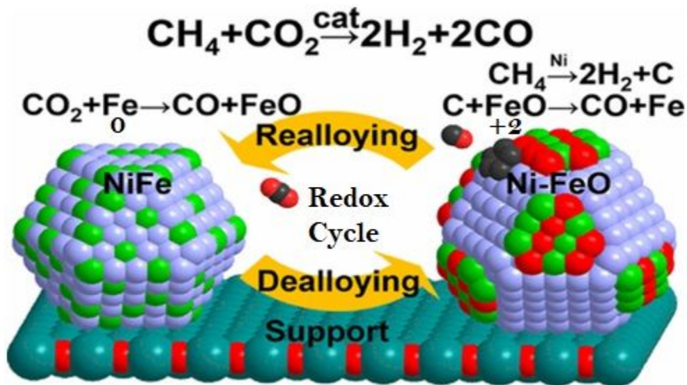
Scheme 3 Dealloying and realloying behavior of an Fe-Ni alloyed particle in DRM modified from 66 .
