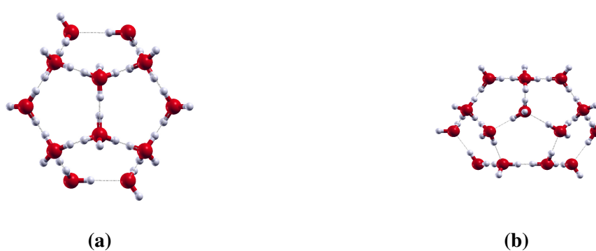
Figure 7.1: Optimized geometries of empty (a) small ( 5^{12} ) and (b) large ( 5^{12}6^2 ) cages of sI clathrate.
