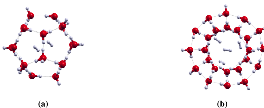
Figure 7.2: Optimized configurations of H 2 molecules at optimum cage occupancies inside (a) small (5 12 ) and (b) large cages (5 12 6 2 ) of sI clathrate.
