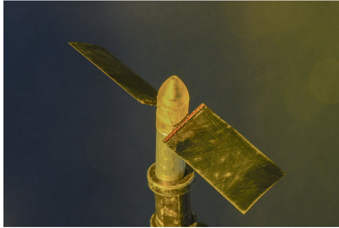
Figure 3.10: Fully flexible propeller, with wider blades
