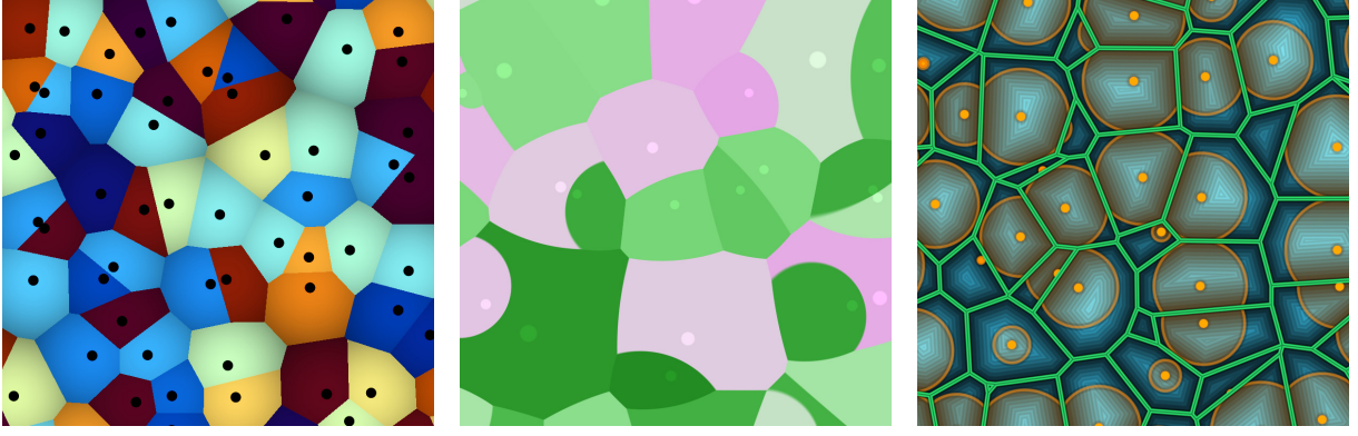
Figure 3.1 – Bidimensional illustrations of a Voronoi decomposition using three types of algorithm: (i) for equally sized circles using the equation 3.1 ( www.shadertoy.com/view/MslGD8 ) (ii) for unequally sized circles using the Apollonian Voronoi decomposition condition 3.2 ( www.shadertoy.com/view/4sd3D7 ) and (iii) another algorithm for unequally sized circles using the radical Voronoi condition 3.3 ( www.shadertoy.com/view/4tV3z3 ). Note that the second picture shows the curved boundaries between the Voronoi cells, while the switch to the radical Voronoi decomposition gives straight line boundaries.
