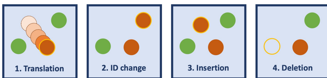
Figure 2.3 – MC moves in a system of two types of monoatomic atoms (green and orange). The modification on the first box is highlighted by the yellow circle and the dragging pattern is represented by a set of dashed circles. The boxes 2 to 4 represent the moves going from the initial state represented in box 1, the corresponding move is highlighted by a yellow outer circle. All these moves are used in the GCMC calculations performed using the RASPA2 software.
