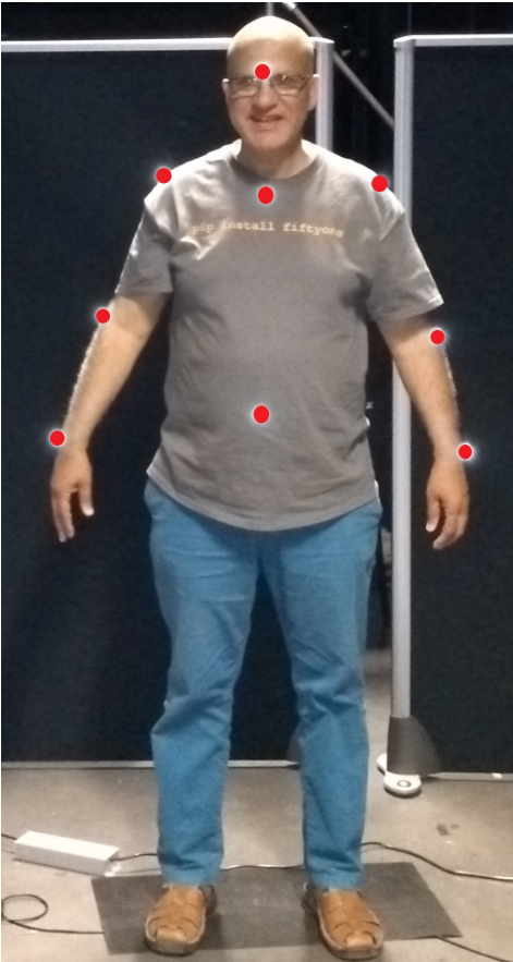
Figure 5.5: Motion capture markers position
