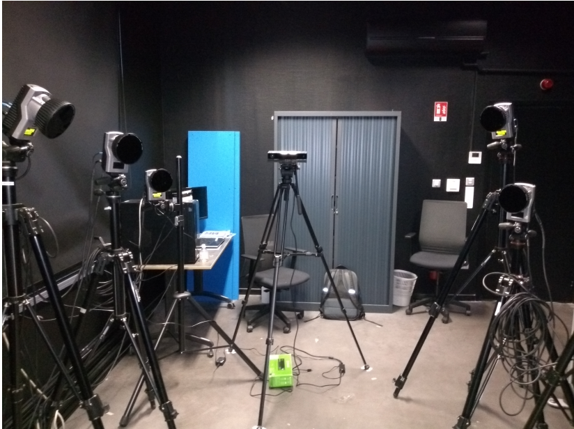
Figure 5.6: Motion capture and Kinect setup. Point of view of the captured subject.
