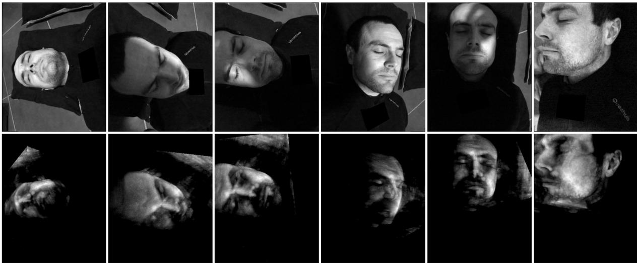
Figure 3.8: Reconstruction with the algebraic technique (3.3), from 72 calibrated images  $384 \times 480$  (see Figure 3.7 for the acquisition). Top: six images of the input sequence. Bottom: MIP “re-projection”. The computation is performed on voxels of size  $h = 1.5$  [mm].
