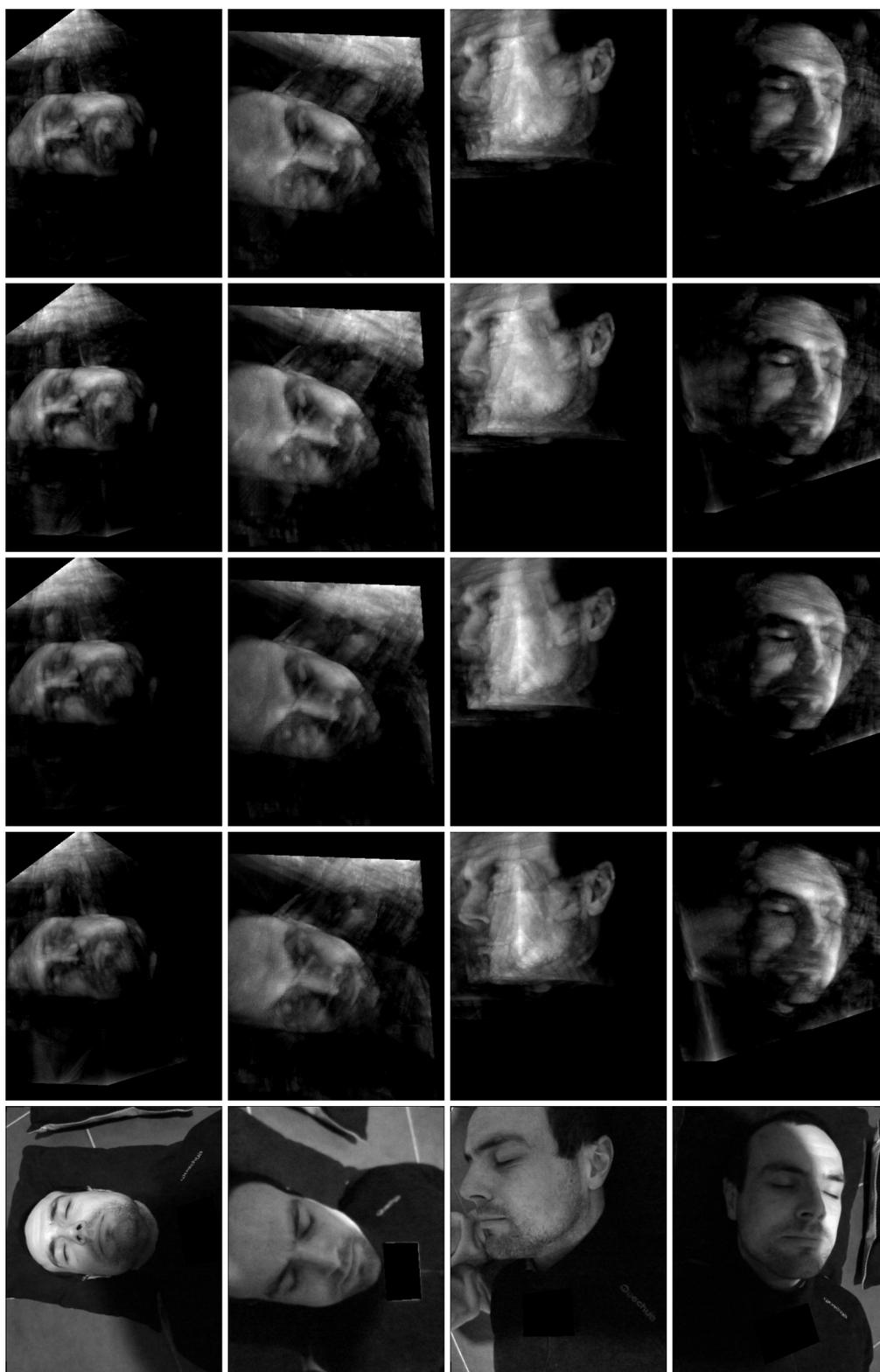
Figure 3.10: Four-fold cross validation of one cycle of algebraic iterations (3.3), from 72 calibrated images  $384 \times 480$  (see Figure 3.7 for the acquisition). A line  $1 \leq i \leq 4$  contains MIP views of the  $i$ 'th reconstruction, trained with 54 images; the views are predictions on the diagonal, re-projections otherwise. The last line contains initial images for visual comparison.
