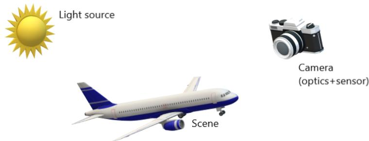
Figure B.2: Image formation in VIS-NIR optics. Light is emitted by light sources and interacts with the illuminated scene. A portion of the light passes through the camera's optics and reaches the camera's sensor.
