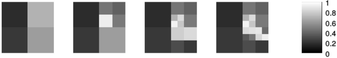
Figure 3.1: Principle of the multiresolution algorithm: compute an image with coarse pixels, then refine sets of bright pixels, iteratively. From left to right: initialization, iteration 1, 2, 3.
