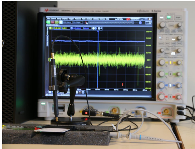
Figure 3.1: EMA , side channel platform of LHS INRIA Rennes.
