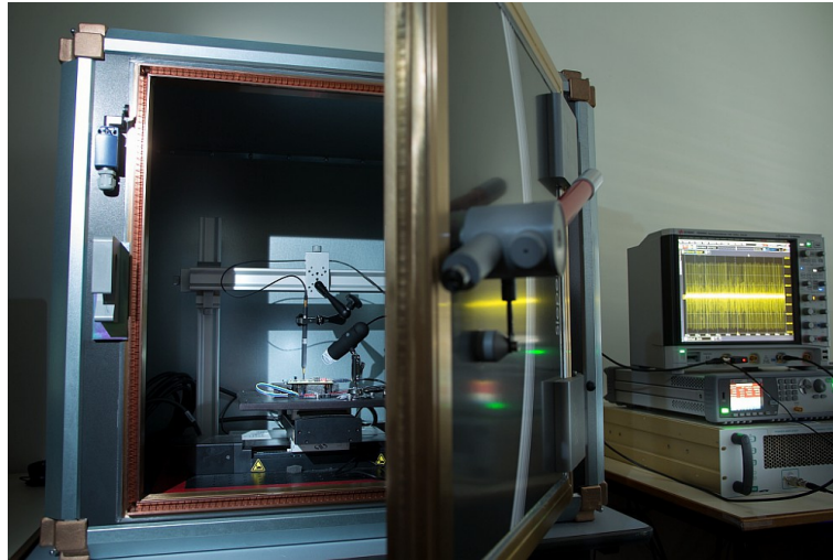
Figure 4.1: Faustine : fault injection bench of the LHS INRIA Rennes. ©INRIA / Photo C. Morel
