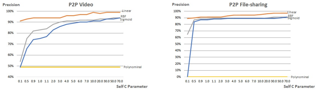
Figure 3.2: Precision, as a function of Self C parameter, of SVM-based classification for P2P video and P2P file sharing traffic.
