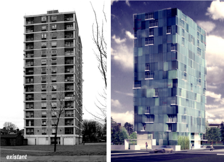
Fig. 30: For the tower block regeneration in London Newham (international competition 2003-04, short-listed project), we proposed adding windowboxes to the facade grafted on the periphery of the building to circumvent costly residents relocation during construction. As a result of the windowbox, the habitability of the dwellings is greatly improved: the surface area is increased, the glass facades bring a massive amount of light inside, and guarantee better thermal and acoustic insulation. Residents co-develop and select windowboxes from a catalogue. The rehabilitation of a low-cost tower block becomes a social and urban catalyst.
