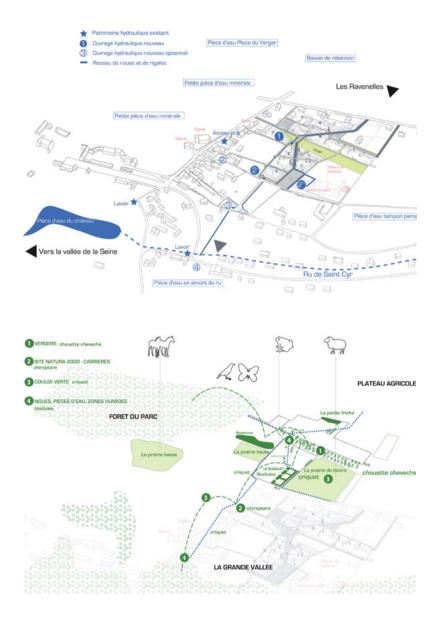
Fig. 41: Ecohamlet - (above) The design of the water system creates spatial qualities for the eco-hamlet and solves the existing drainage problems of the village; (below) A differentiated management supports the ecological corridors of the wider landscape.
