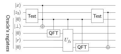
Figure 3.1: A quantum circuit implementing our CFourierO<sub> $f_2 \circ h$ </sub> oracle. Depending on the control bit b which is the output of Test, if b = 1, we apply  $U_{f_2}$ , otherwise, we apply the identity. The bit b will be discarded after the computation.
