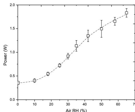
Figure 21 - Evolution of the plasma injected power as a function of air relative humidity (RH). The applied voltage and frequency are fixed as 10 kV and 1000 Hz. The injected power was measured by (q-V) Lissajous Method.
