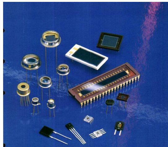
Fig. 2.18 Picture of photodiodes with different shapes and size (Hamamatsu HPK)
