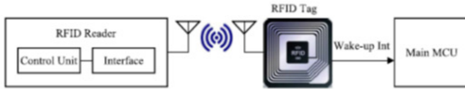
Figure 2.10: RFID Wake-Up Radio based prototype [45]
