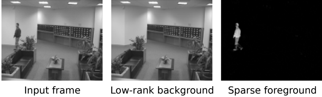
Figure 2.3: Robust Principal Component Analysis (RPCA) applied to a video frame. We see that the low-rank background and the sparse foreground are simultaneously retrieved using RPCA. Results taken from [42].
