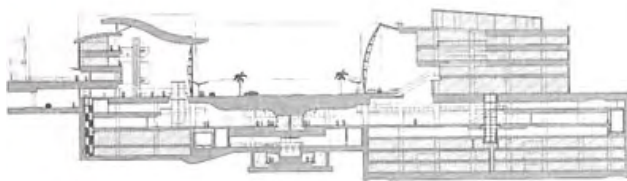
cross section of complete scheme, with stage II (hotels and retail, on right – north)
