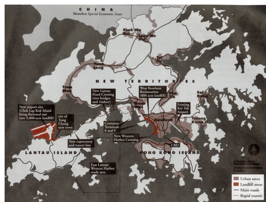
The Airport Core Program includes a new airport, new port facilities, new road and rail links, and more than 3,000 acres of landfill.
