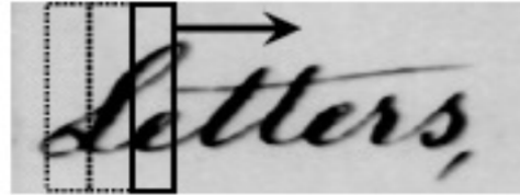
Figure 2.11: Use of a sliding window for extracting small fragments.
