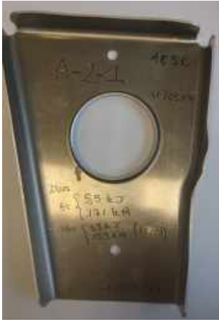
Figure 2.13: AA1050 formed part. Extracted from [159].
