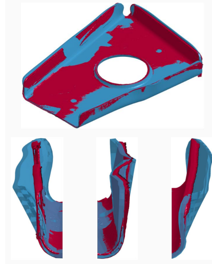
Figure 2.14: Superposition of the computed (in blue) and measured (in red) deformed shapes. Extracted from [159].
