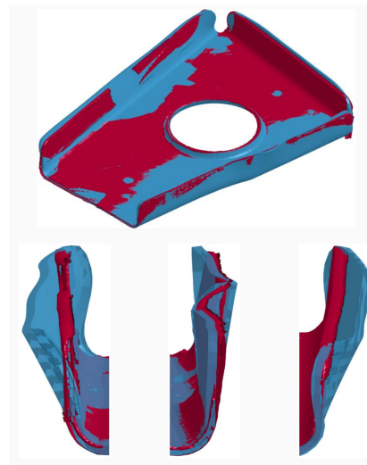
Figure 2.14: Superposition of the computed (in blue) and measured (in red) deformed shapes. Extracted from [159].
