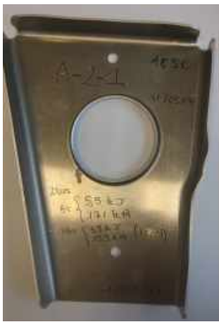
Figure 2.13: AA1050 formed part. Extracted from [159].
