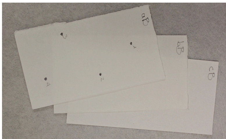
Figure 3.1. Ruscombe Paper Mills paper: the four points where thickness was measured on each sample are marked with a pencil mark.
