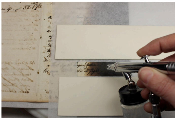
Figure 1. Distribution of the reinforcing formulation MFC/CNC/TEOS by airbrush on the charred area of the manuscript from the 19 th century.
