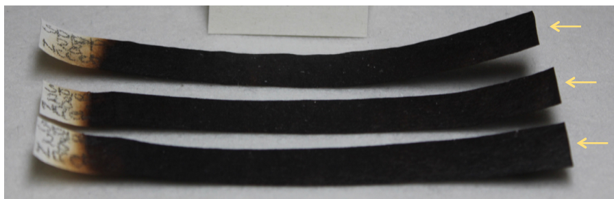
Figure 5.3. Deformation of sized RPM sample treated recto/verso with the 0,3% w/v CNC dispersion in ethyl alcohol.
