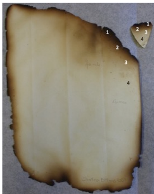
Figure 2.21. The historical sheet belonging to the manuscript from Chartres and a triangular-shape fragment from the Padua incunabulum (left, in evidence the different bunt areas numbered 1,2,3 and the unburnt area 4).
