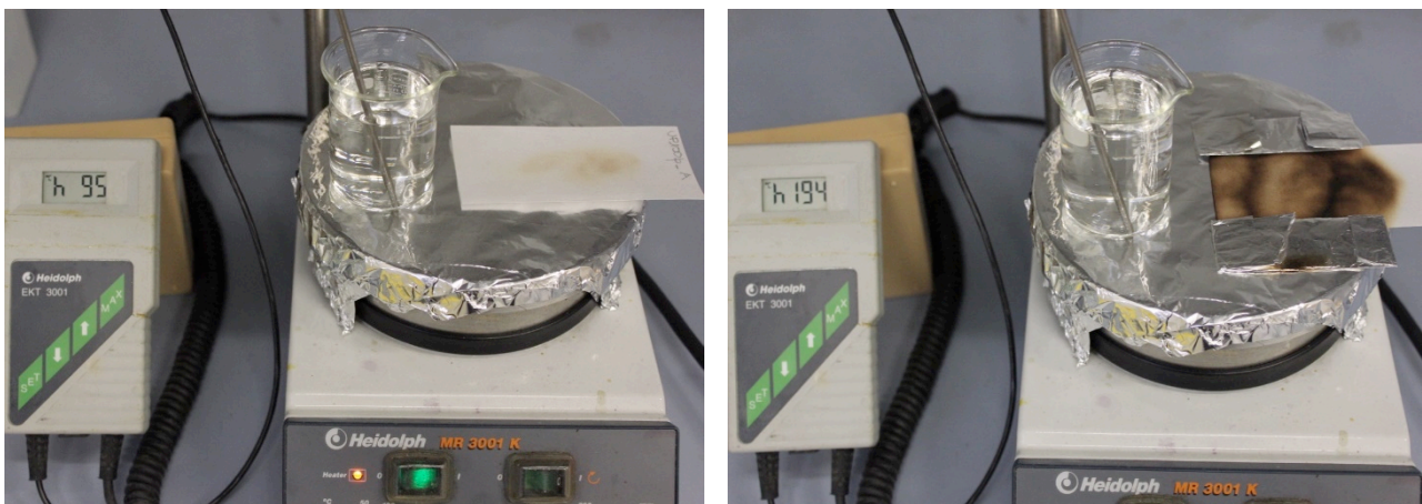
Figure 3.5. Progression in the burning process of unsized RPM sample from 95° to 194°C.
