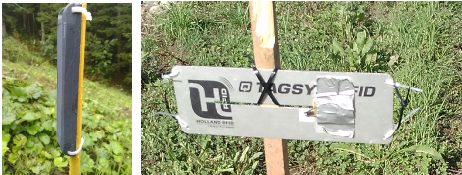
Figure A-8: (left) Survivor B tag, a metal-mount tag with a patch antenna, and (right) a prototype of tag with a higher gain provided by Mojix, using a slot antenna coupled with a magnetic loop.
