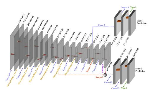
Figure 5.11: Tiny-YOLOv3 network Architecture (redrawn from [151])
