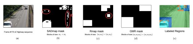
Figure 5.2: ROI construction and GMR mask use for extra blocks elimination.
