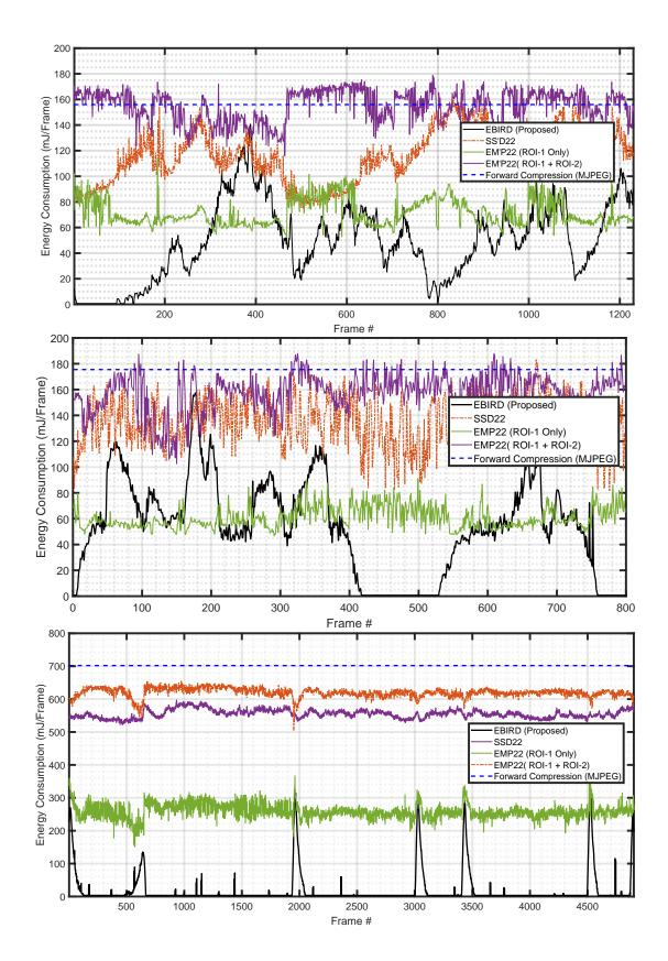
Figure 3.6: Per-frame energy dissipation of BIRD for Highway, pedestrians and Snowfall
