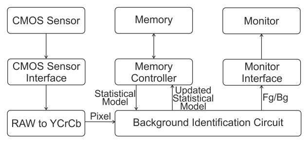
**Figure 1.4:** A conceptual example of background modeling circuit embedded in FPGA board (redrawn from [61])
