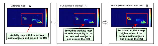
Figure 3.3: Impact of the combination of FGS and ROF on the ROI classification
