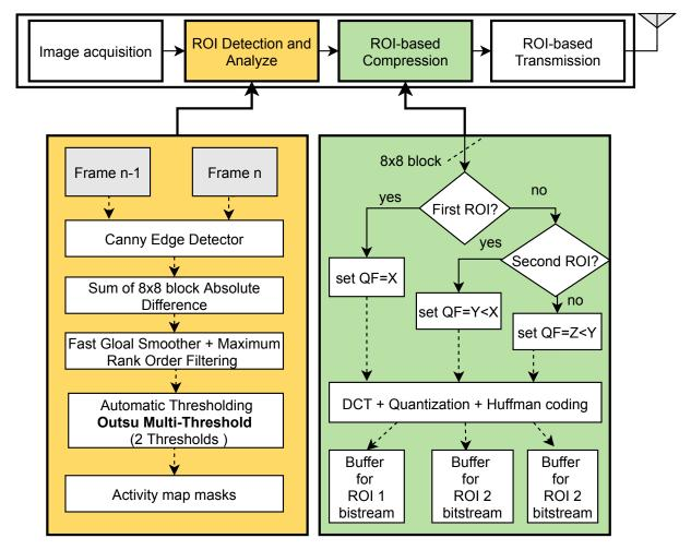
Figure 4.1: Proposed ROI-based video compression scheme
