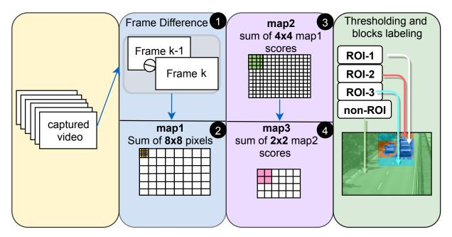
**Figure 5.3:** The proposed scheme illustration with  $w_1 = 8$ ,  $w_2 = 4$  and  $w_3 = 2$ .
