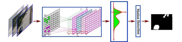
Figure 1.5: Wavelet-based background modeling for MOD proposed in [58].
