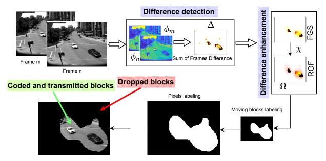
Figure 3.1: Block diagram of the proposed algorithm (BIRD)
