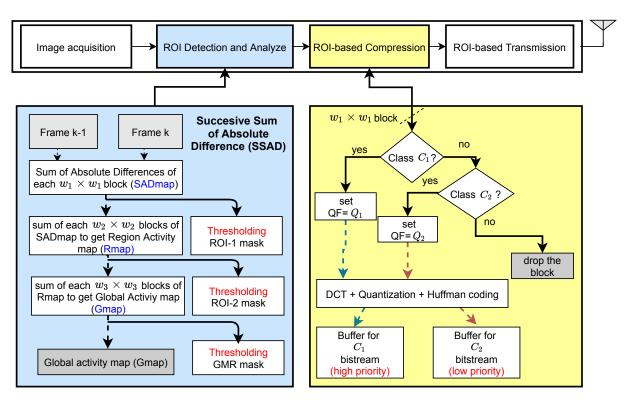
Figure 5.1: The scheme of the proposed strategy for a 3-level ROI-based video coding.
