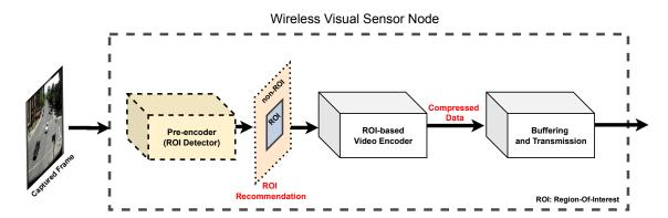
**Figure 1.9:** A sensor node employing ROI detection as a pre-processing step before compression
