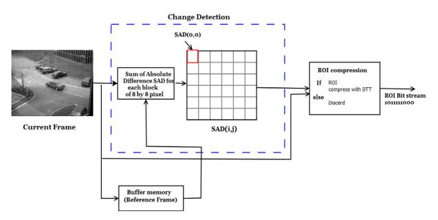
Figure 1.6: ROI detection and coding approach proposed in [64].
