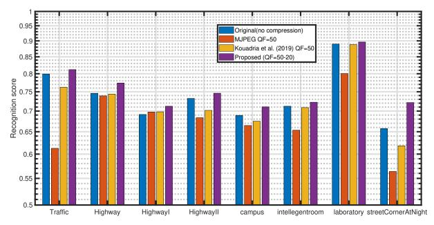
Figure 5.13: Performance of recognition: Recognition accuracy
