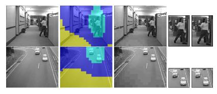
**Figure 4.3:** Results of multi-QF based coding. from left to right: 1- Original Frame 2- Segmentation Results 3- Decompression results (JPEG chain with ROI1: QF=90, ROI2:QF=50, ROI3:QF=10 - PSNR=33.9308, SSIM=0.7618) 4- ROI visual quality for same bitrate(proposed left, MJPEG right).
