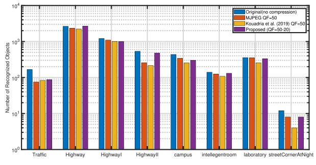
Figure 5.12: Performance of recognition: Number of detected objects
