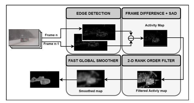
Figure 2.2: Block diagram of the proposed ROI Detection.
