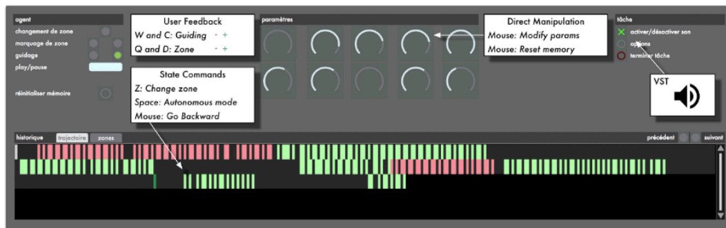
Figure 13 Co-Explorer Interface (image adapted from (Scurto et al., 2021)). On the top left, the interface depicts the user feedback controls (such as 'like' or 'don't like', or 'change zone'). At the top centre, a user could manipulate directly the parameters structuring the design space. At the bottom, a timeline shows the progression of the learning phase and depicts the previous interactions (e.g. a green bar refers to positive feedback from the user).
