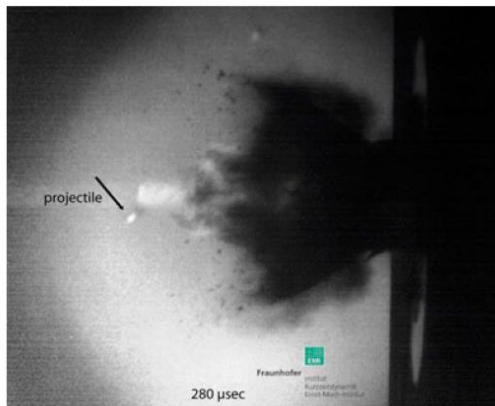
Fig. 3. High-speed shadowgraph image of dry experiment P1-2808, showing a reflected projectile relic (black arrow indicates bright particle) as it overtakes the central plume. The brightness indicates a high temperature.
