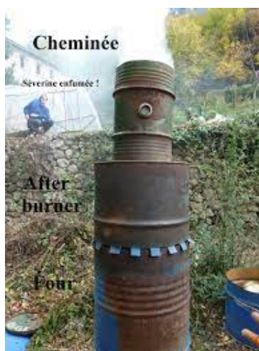
FIGURE 1.5 – Four de carbonisation [14]
