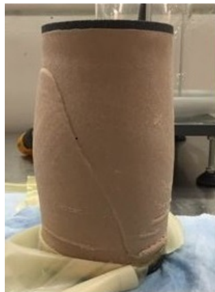
Figure 2.2: Shear band formation in a cylindrical specimen [10].
