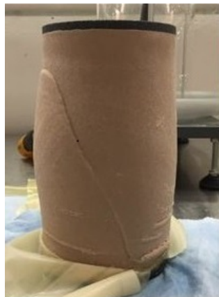
Figure 2.2: Shear band formation in a cylindrical specimen [10].
