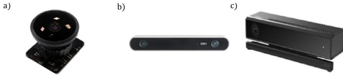
Figure 2.12: Examples of monocular camera (a), stereo camera (b) and RGB-D camera (c) (adapted from Y. Lu et al., 2018 [144]).
