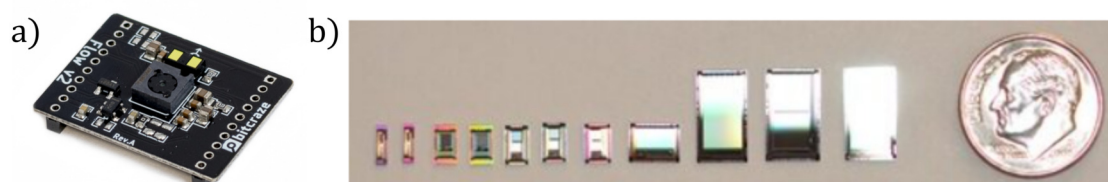
Figure 3.10: Examples of (a) optic flow sensor (PMW3901 model by PixArt Imaging Inc., [117]) and (b) vision chips (by CentEye Inc. [116]).
