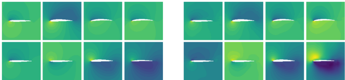
Figure 4.27: A set of predictions on flow field Pressure from Out-of-Distribution Test Set . Left: Simulation by OpenFOAM (Ground Truth), Right: Prediction from Graph U-Net
