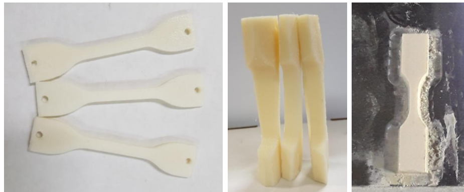
(a) ABS normalized specimen
