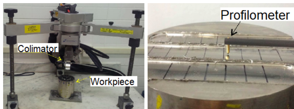
(c) Residual stress and roughness measurements
