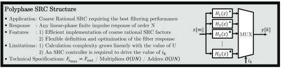
Figure 3 Fundamental SRC: U-F-D and polyphase structures.
