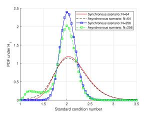
**FIGURE 9.** Probability density function of the SCN under  $\mathcal{H}_1$  as function of N with M=1024 and SNR = 0dB.
