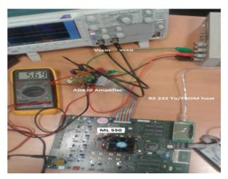
Figure 6.7 – Power measurement setup.
