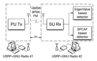
Fig. 1. Schematic system diagram
