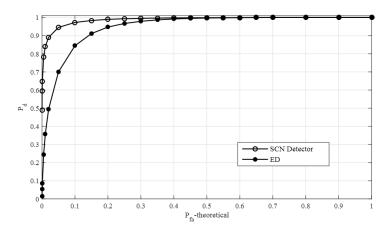
Figure 5.6 – ROC of the SCN-based detector vs. ROC of the ED where K=3, N=500, SNR=-10 dB and 0.1 dB of noise uncertainty.
