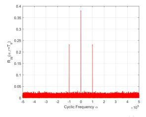
Figure 5.4 – Magnitude of cyclic auto-correlation function  $\hat{R}_{yy}^{(\tau)}(\alpha)$  at  $\tau_0 = T_s$  for a BPSK modulated signal and SNR = -3 dB where  $T_s$  is the sampling period.
