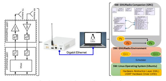
Figure 6.12 – USRP hardware platform and GNU Radio software architecture.
