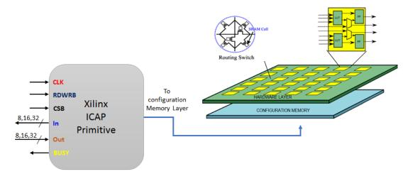
Figure 6.5 – The ICAP primitive on Xilinx FPGAs.
