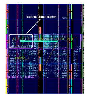
Fig. 4. Placement of top-level modules.
