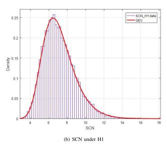
Fig. 12. SCN measurements and PDF fitting curves,  $\rho = -10 dB$ , K = 4, N = 500.
