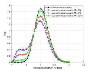
**FIGURE 8.** Probability density function of the SCN under  $\mathcal{H}_1$  as function of M with N=128 and SNR = 0dB.
