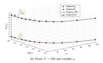
Fig. 6. Empirical  $P_{fa}$  and  $P_d$  of the SLE detector and its corresponding target values by using dynamic method.
