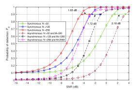
FIGURE 10. Probability of detection versus SNR with target false-alarm probability equal to 0.1, and different (N, M) pairs.
