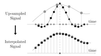
Figure 4 Example order 3 interpolation of an up-sampled signal.
