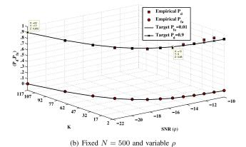
Fig. 2. Empirical  $P_{fa}$  and  $P_d$  of the LE detector and its corresponding target values by using dynamic method.
