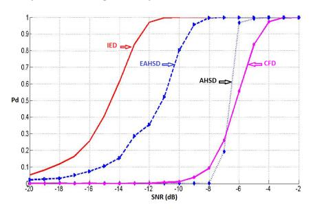
Figure 5.3 – Detection performance for IED, CFD, AHSD and EAHSD detectors with  $P_{fa}=0.01$ .
