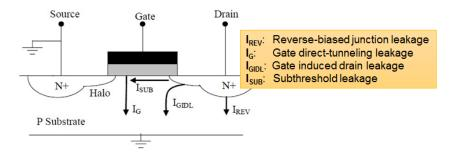
Figure 6.8 – Main CMOS leakage currents.
