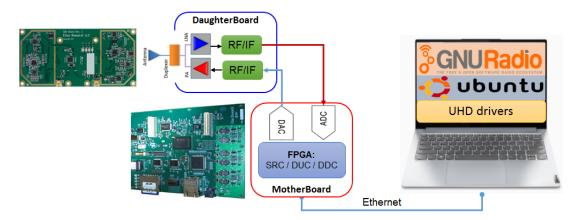
Figure 6.11 – GPP-based SDR platform (Ettus USRP N210 board & GNU Radio framework).
