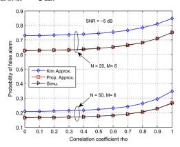
Fig. 4. Probability of false alarm  $P_{fa}$  plotted against correlation coefficient  $\rho$  values for SNR =-5 dB and  $P_d=0.99$ .
