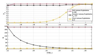
Fig. 5. Empirical  $P_d$  of the SCN detector and the corresponding number of antennas, K, used for sensing in Full, Dynamic and Fixed methods w.r.t  $\rho$ and fixing N = 500.
