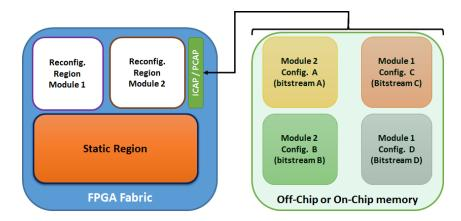
Figure 6.4 – Dynamic Partial Reconfiguration scheme.
