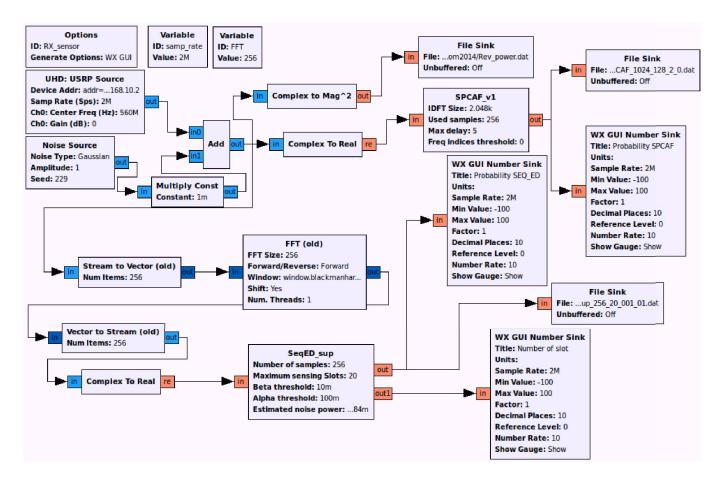
Fig. 5. Diagram of the SU receiver realized in the GNU radio (Screenshot from GRC)
