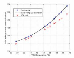
Fig. 3. Leakage currents consumption versus FPGAs fabric temperature.
