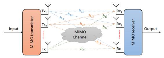
Figure 4.1 – Wireless MIMO system with t transmitter and r receiver antennas.
