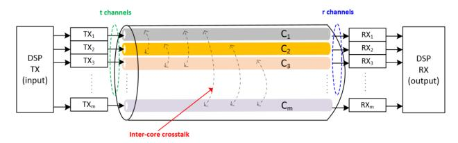
**FIGURE 1.** Schematic of an optical MIMO system with an MCF,  $C_k$  indicates  $k^{th}$  fiber core, with  $k \in \{1, 2, ..., m\}$ .
