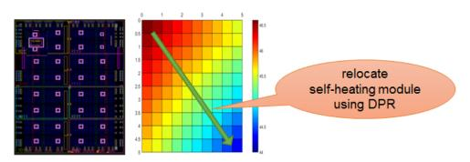
Figure 6.10 – Thermal map of Virtex-5 (65 nm) obtained using an uniform interpolation of RO sensors responses.
