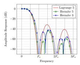
Fig. 4. Frequency responses of Lagrange and Hermite interpolations
