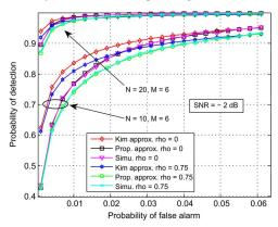
Fig. 3. Receiver operating characteristics (ROC) curves for the two approximations at SNR  $=-2~\mathrm{dB}$ .
