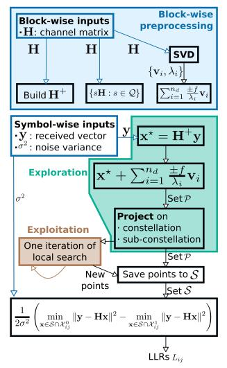
FIGURE 5. Summary of the proposed new geometrical detector.
