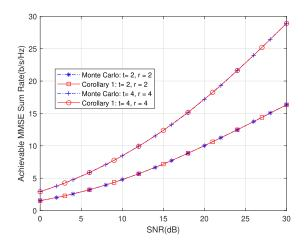
FIGURE 7. Evolution of the ergodic sum rate for the MMSE receiver over an uncorrelated MIMO Rayleigh fading channel.
