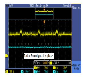
Fig. 6. FPGA core power consumption during partial reconfiguration
