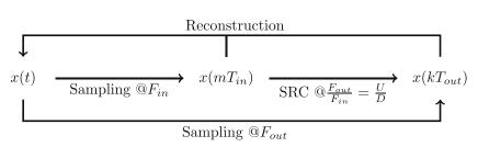
$2 \times f_m$  [11]. Sampling rate conversion is then defined as the operation that takes the samples  $x(mT_{in})$  as input, and outputs  $x(kT_{out})$ , with the change in the sampling frequency defined by the SRC factor R:
