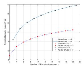
FIGURE 5. Ergodic capacity of MIMO Rayleigh channel when the number of received antennas increases and ho= 10 dB.
