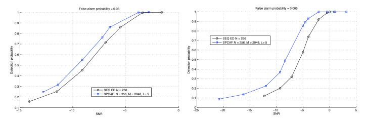
Fig. 6. Probability of detection for both algorithms when using FM signal as PU  $(P_{fa}=0.08)$
