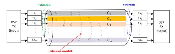
Figure 4.2 – Optical MIMO system with an MCF,  $C_k$  indicates  $k^{th}$  fiber core, with  $k \in \{1, 2, ..., m\}$
