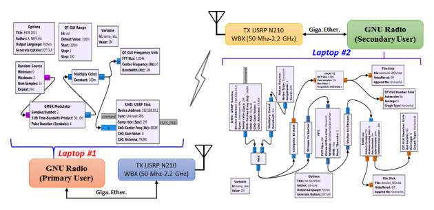
Figure 6.13 – A simplified block diagram of sensing performance measurements with GRC flow-graphs associated to PU and SU equipments.
