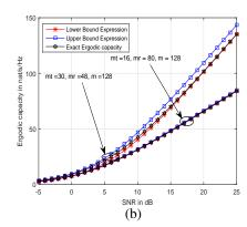
Fig. 2. (a) Low-SNR upper-bound approximation of the ergodic capacity in nats per channel use versus SNR in dB, (b) Bounds and simulation results for ergodic capacity of MIMO Jacobi channel capacity, with number available modes m = 128, for different numbers of transmitting and receiving channels.
