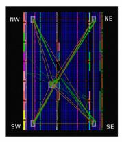
Fig. 1. Thermal sensors' position inside the FPGA.
