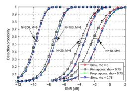
Fig. 2. Probability of correct detection plotted against SNR values.
