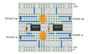
Fig. 3. AD620 amplification circuit.
