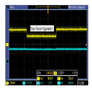
Fig. 5. FPGA core power consumption during total reconfiguration
