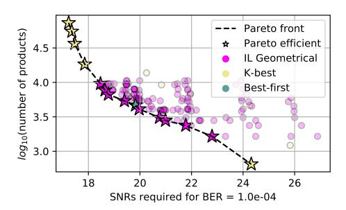
Figure 4.5 – Complexity vs. performance trade-off, Pareto plot compares the lowest required SNR (horizontal axis) versus the lowest complexity in the number of product operations (vertical axis) for  $4 \times 4$  coded MIMO system with 16-QAM using IL Geometrical, soft-output K-best sphere decoding and soft-output Best-first sphere decoding algorithms.
