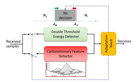
Figure 5.2 – Block diagram of hybrid spectrum sensing detector.
