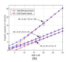
Fig. 1. (a) Comparison of the ergodic capacity and analytical lower-bound and upper-bound expressions for  $(m_t = m_r = 2, m = 6)$ , and  $(m_t = 4, m_r = 10, m = 16)$  uncorrelated MIMO Jacobi-fading channels, (b) High-SNR lower-bound approximation of the ergodic capacity in nats per channel use versus SNR in dB.
