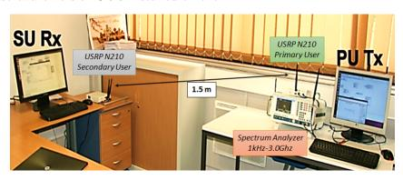
Figure 6.14 – Experimental setup for spectrum sensing using GNU Radio and USRP devices.
