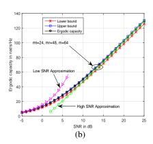
Fig. 3. (a) Comparison of upper bound, lower bound and ergodic capacity in nats per channel use versus SNR in dB when  $m_t + m_r$  is larger than the available modes m (b) Bounds, upper and lower SNR approximation of the ergodic capacity of the MIMO Jacobi-fading channel where the number of available modes m = 64 and  $m_t + m_r > m$ .
