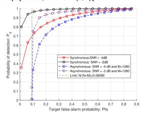
FIGURE 11. The ROC curves for N=128. Solid lines represent different SNR values, -4 dB and -2 dB, under synchronous PU traffic, dashed lines represent different SNR values, -4 dB and -2 dB, under asynchronous PU traffic for fixed  $M=10 \times N$ , and dot-dashed line represent the theoretical lower bound of false-alarm probability under asynchronous scenario with N=128 and M=1280.
