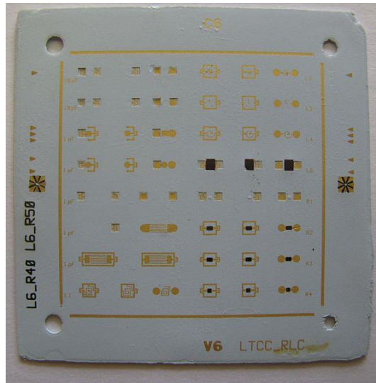
Figure 42. The RLC prototype containing MIM and interdigital capacitors, spiral inductances and resistances [40]
