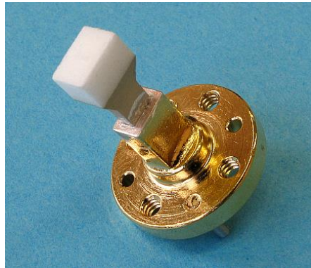
Figure 29. Origin 60-GHz horn antenna realized in silver painted Rohacell™ foam, produced in-house
