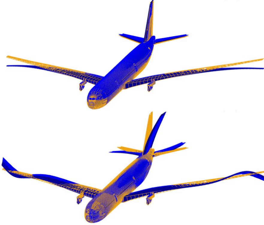
Figure 2.10: First bending (up) and torsion (down) modes shapes of the XRF1-HARW
