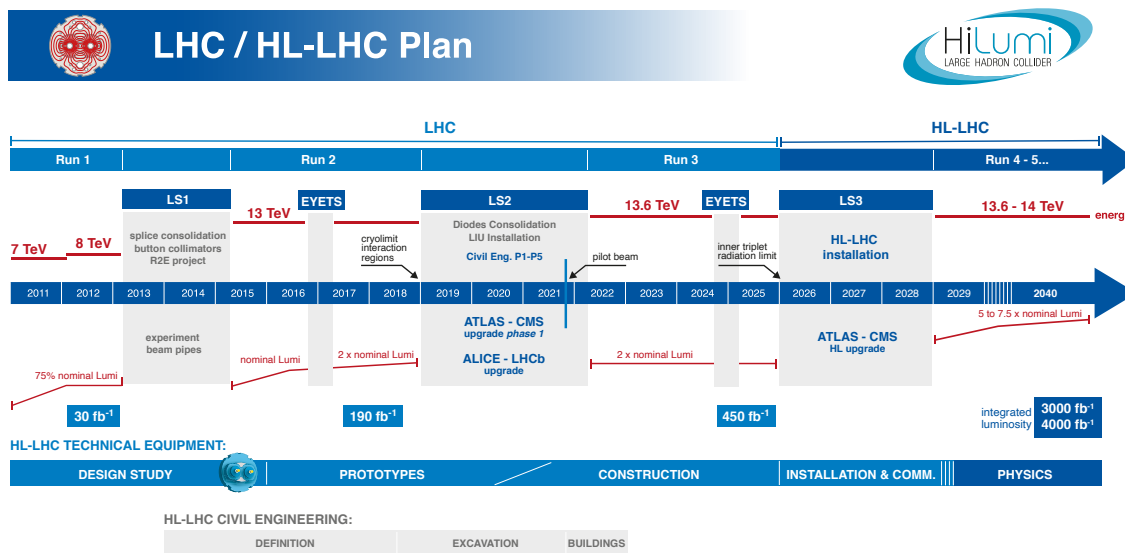
Figure 2.8.: CERN's upgrade path towards the High-Luminosity LHC (HL-LHC) [52].
